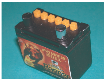
A car battery contains 6 cells.
