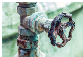
Can you see the green coating forming on this copper tap?
