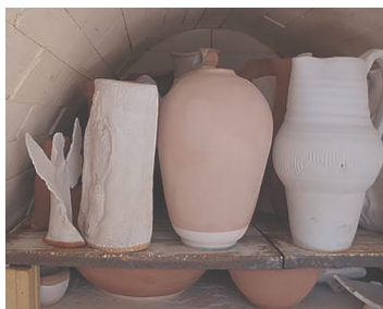
These clay pots have been dried and they have just been loaded into a kiln to be fired. 3
