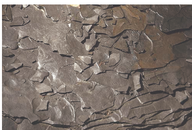
Shale splits easily into thin tiles which can be used in flooring and roofs. 13
