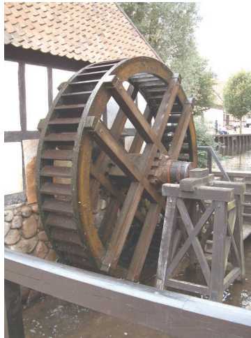
A water wheel uses the flow of water to push the wheel around, which can then do work.
