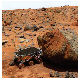
This is the rover that was carried by the Pathfinder spacecraft. It has instruments to find out what the rock is made of.
