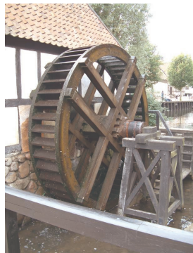
A water wheel uses the flow of water to push the wheel around, which can then do work.
