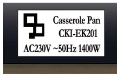
Figure 19.1: The label on an electric pan indicating a power rating of 1400 W.
