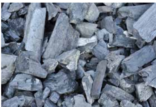
Figure 22.21: Lumps of coal can be used directly as a fuel. However, some coal is first washed to make it into 'high-grade coal'. It can also be sorted into various sizes, depending on what the fuel is required for.
