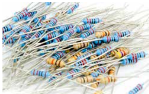
Figure 15.2: Different types of resistors are used to add resistance to an electric circuit.
