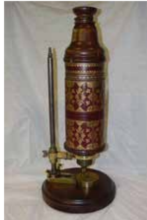
Figure 1.3: Robert Hooke's microscope that he used to view cells for the first time.
