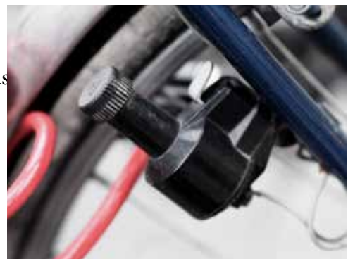
Figure 18.13: A dynamo on the wheel of a bicycle.
