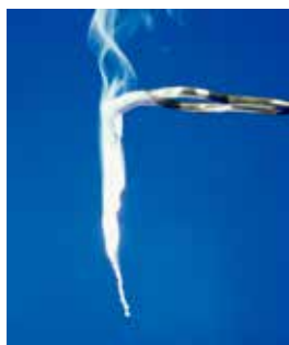
Figure 8.2: Magnesium burns with a bright white flame.
