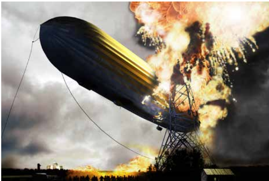
Figure 9.9: In 1937, a German airship exploded and fell to the ground in a huge fireball as the hydrogen gas which kept it floating ignited and reacted with the oxygen in the air.
