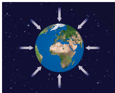
Figure 13.14: The arrows show the direction of the gravitational field of the Earth. The arrows all point towards the centre of the Earth because the gravitational force is always attractive
