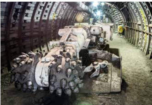
Figure 22.11: A machine called a continuous miner at work at the coal face.
