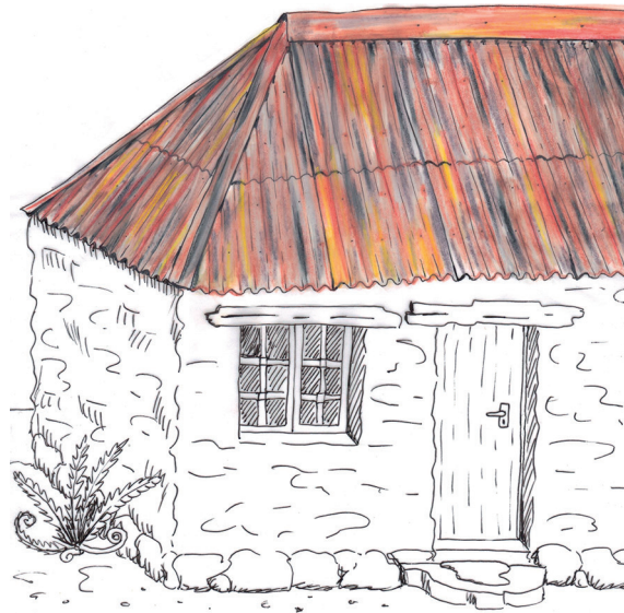
Figure 5: The coating of zinc has worn off this corrugated steel roof.
