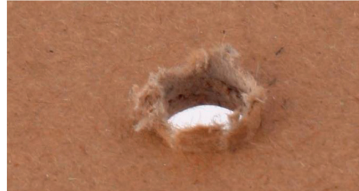
rough side of a punched hole
