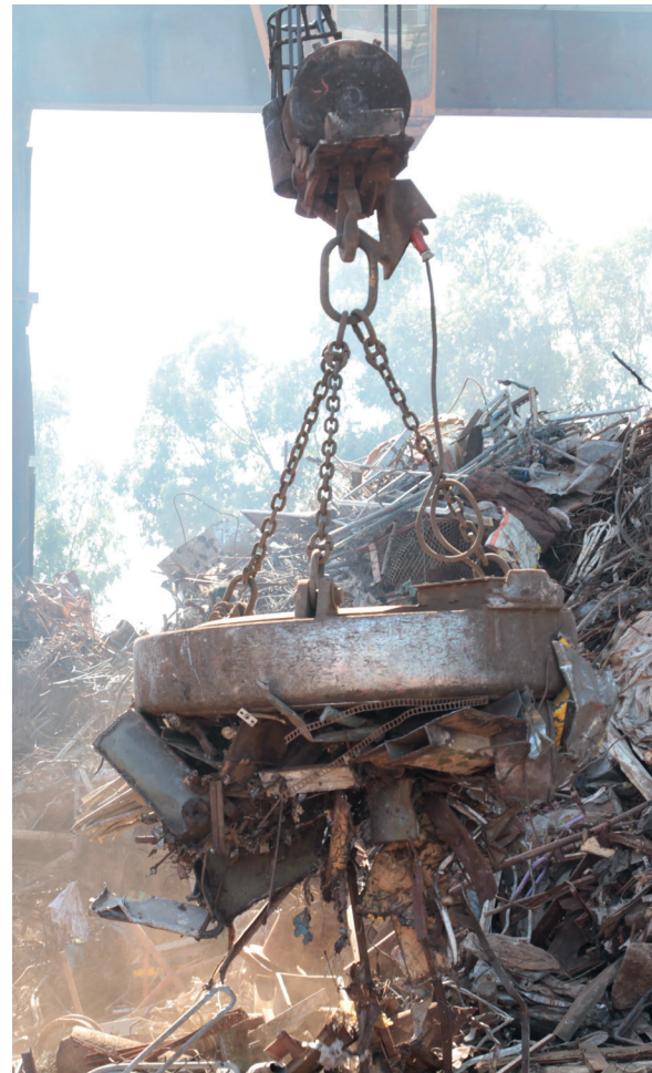
Figure 6: An electromagnet is used to sort metal in a scrap metal yard.
