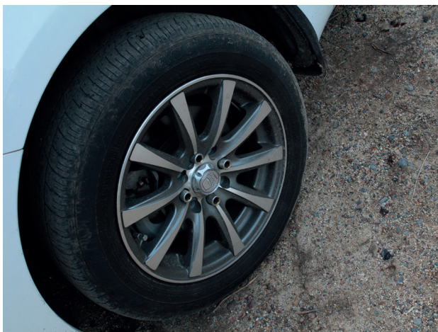
Figure 13: A rubber tyre is a shell structure.
