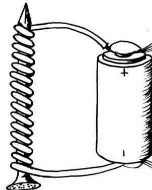
Figure 7: A simple electromagnet
