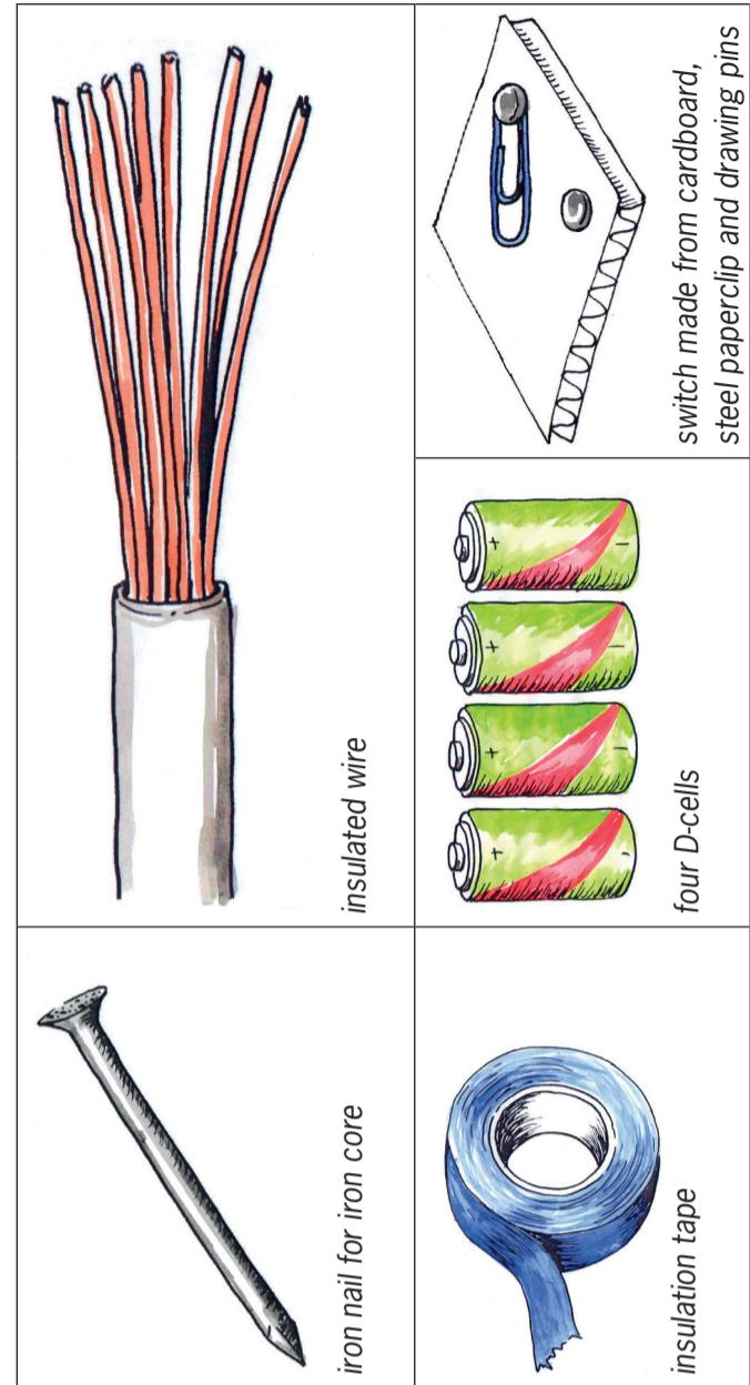
Figure 19: Materials used to make an electromagnet
