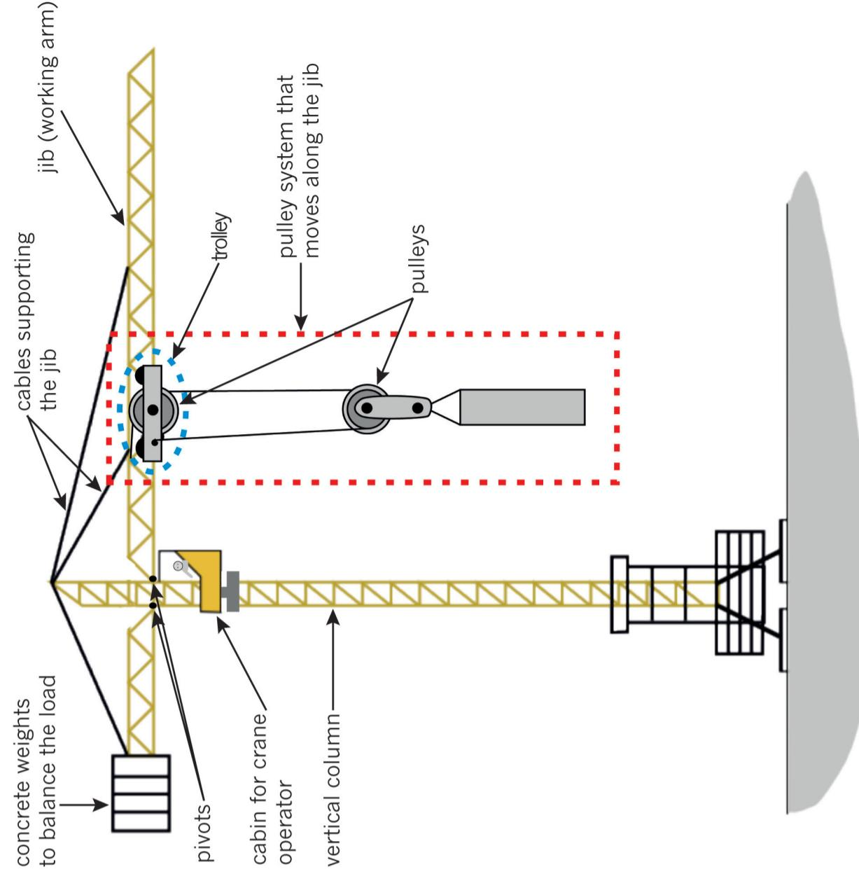
Figure 3: A tower crane uses many different mechanisms.
