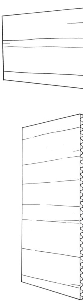
Figure 2: These pictures show two corrugated cardboard sheets of about 20 cm long and 10 cm wide. The one piece has the corrugations over the width, and the other piece has the corrugations over the length.
