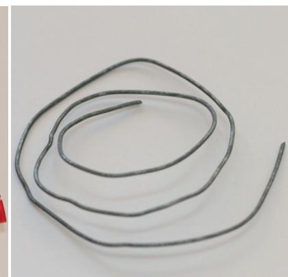
Galvanised steel, wire 1 mm (optional: if pliers or other tools for cutting and bending wire are available)
