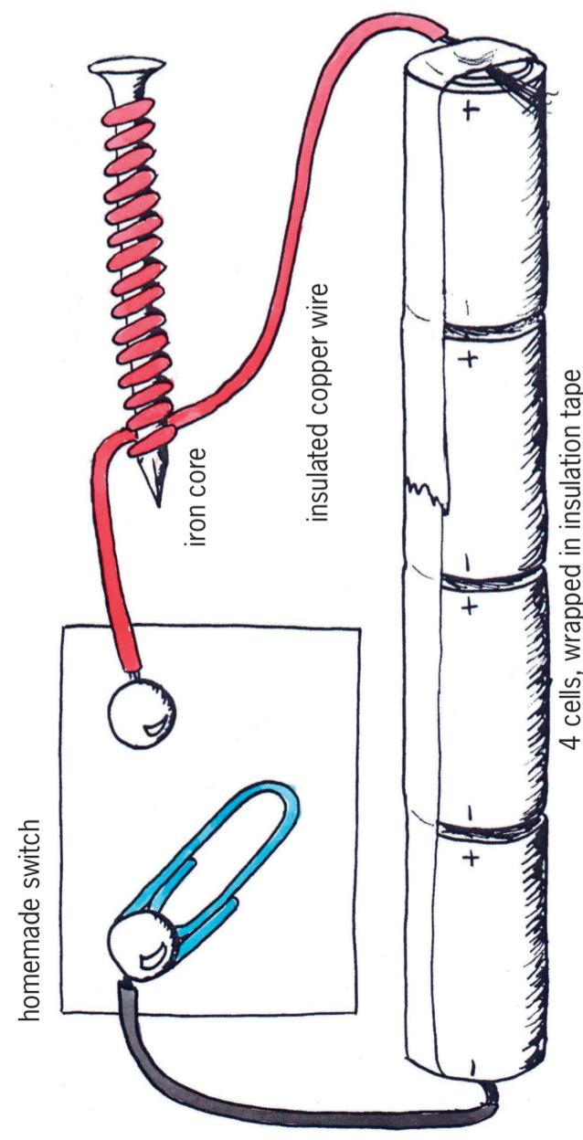
Figure 20: Electromagnet
