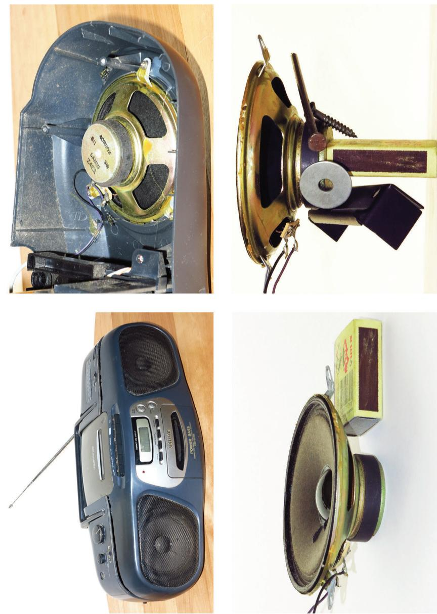
Figure 1: The back of a speaker can be used to pick up certain items!
