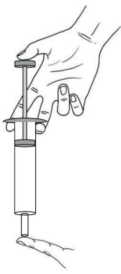
Figure 7: Close the outlet tube tightly with a finger, then try to push the plunger in.
