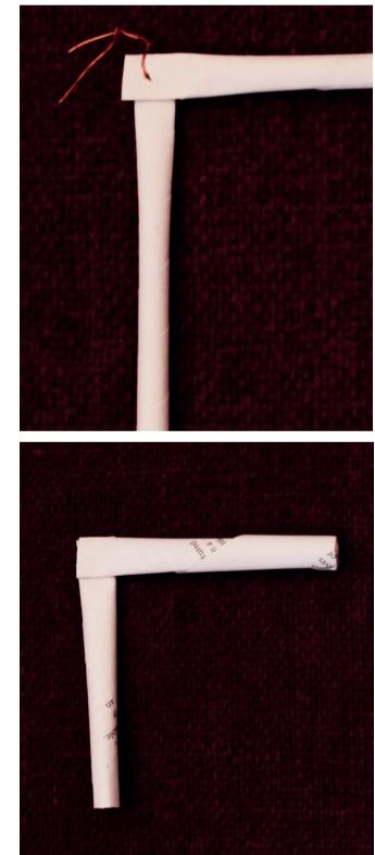
B. Joining two straws by pasting C. Using wire to make a joint with glue
