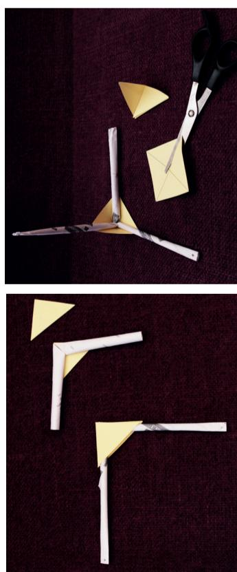
E. Making and using triangular card gussets to strengthen a joint
