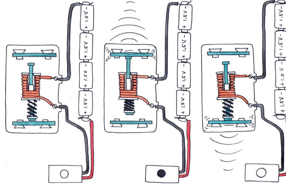
Figure 1: How does an electric door bell work? The coiled copper wire of an electromagnet forms part of the electric circuit.
