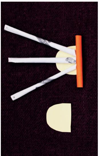
D. Using a card gusset to strengthen a joint
