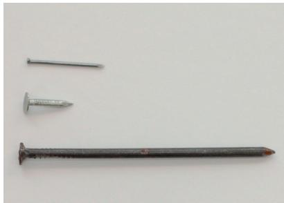
Nails (1 mm, 2 mm, 4 mm, and 6 mm diameters; minimum lengths between 3 cm and 8 cm)
