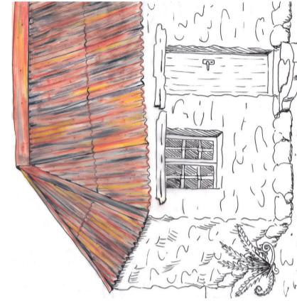
Figure 5: The coating of zinc has worn off this corrugated steel roof.
