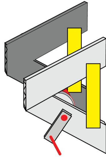
Figure 12: Put your crank and winder into your A-frame.
