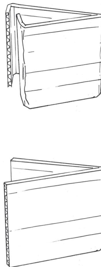
Figure 3: Both pieces are folded in the middle to form springs. The edges are folded to form flanges.
