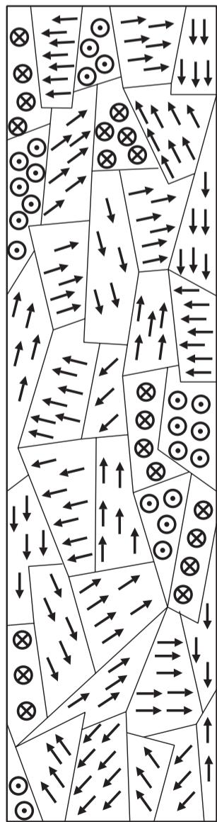
Domains inside a bar of iron. Notice that the domains are magnetised in different directions.
