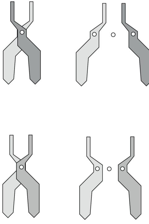
Figure 1: A set of pliers consists of two levers that pivot/rotate around the same fulcrum.
