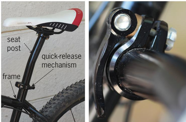
Figure 12: A quick-release mechanism is used to clamp the seat post to the frame of this bicycle.
