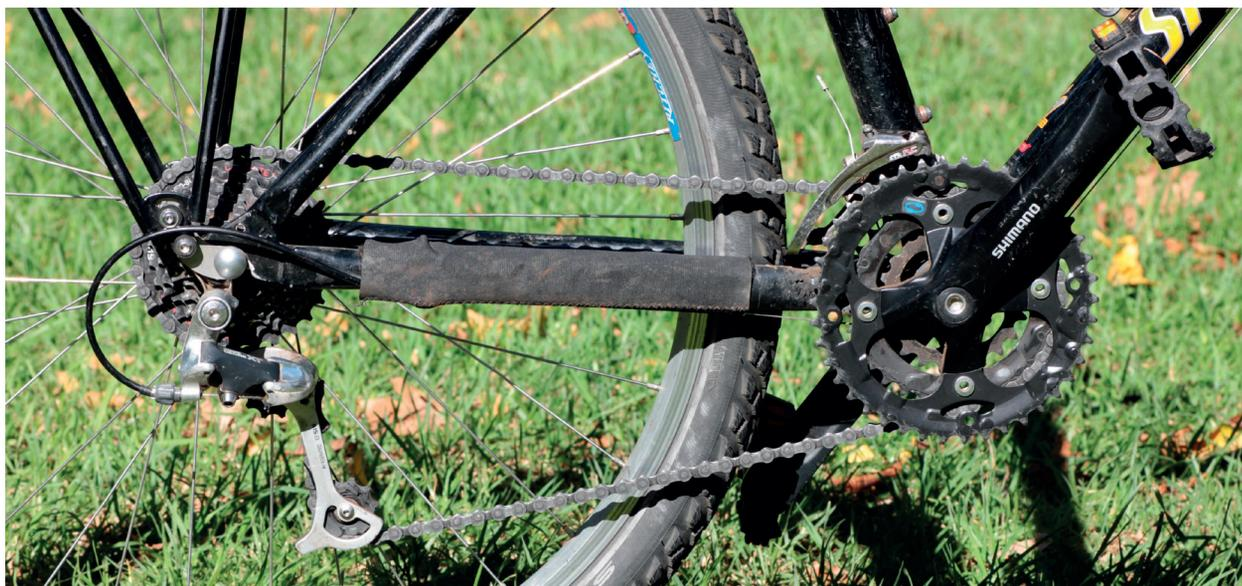
Figure 1: A photograph of the chain drive of a bicycle
