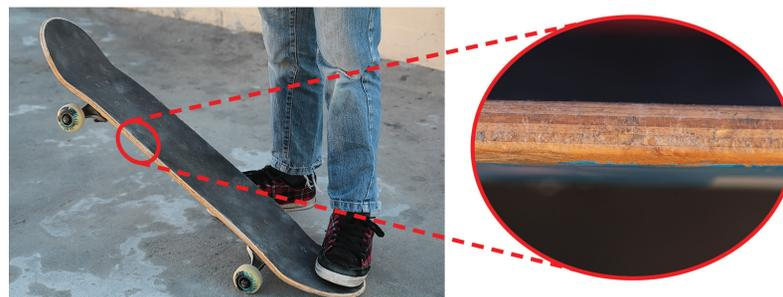
Figure 23: A skateboard is made of plywood
