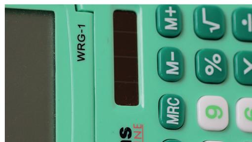
Figure 15: Photovoltaic cells in a calculator
