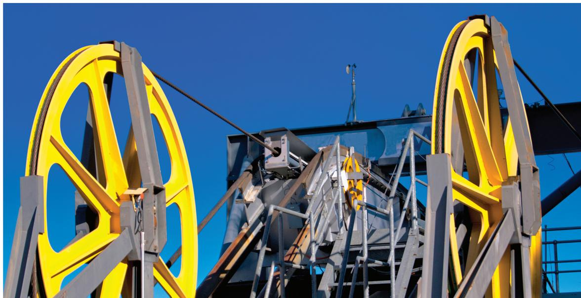
Figure 2: This photograph shows detail of sheave wheels used for pulling in a cable. The sheave wheels in the photograph are used for a cable car, but they are similar to the sheave wheels used on a mine’s winch system.
