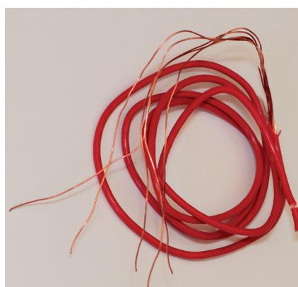
Copper wire, 1 mm (this bends easily by hand and can be cut with scissors; buy from hardware store)
