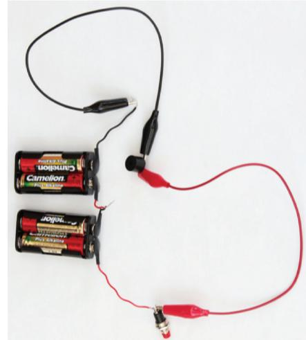
Figure 2: A simple doorbell circuit
