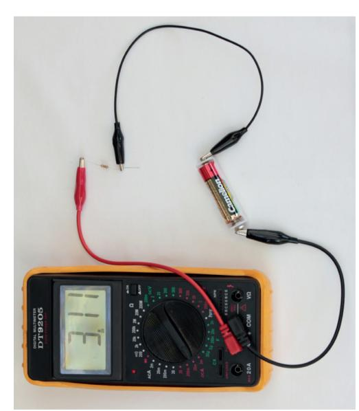
Figure 18: Multi-meter set and connected to measure current
