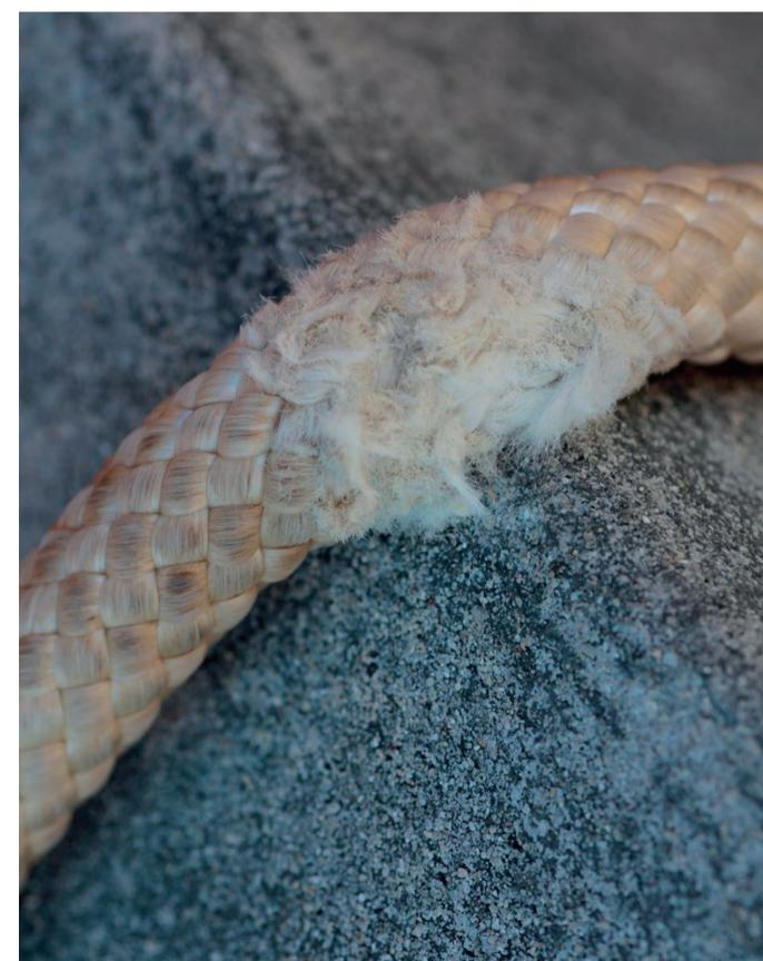
Figure 3: This rope has been rubbed against the edge of a brick.
