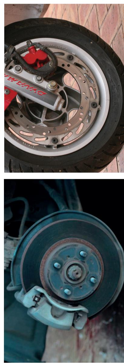
Figure 18: Disc brake on a car
