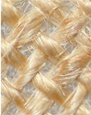
Figure 2: Close-up photo of plant fibres that were spun and woven to make a fabric
