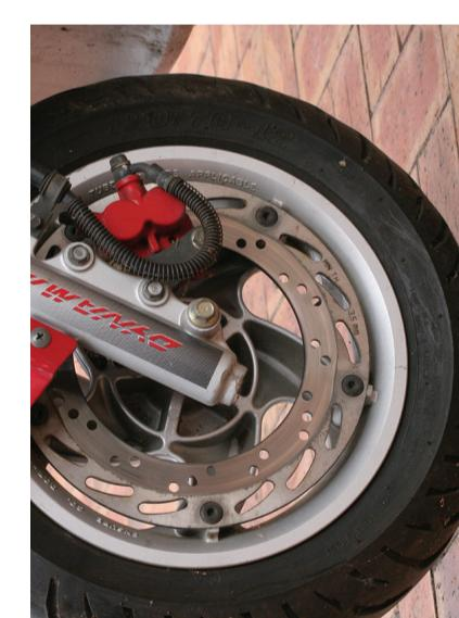
Figure 19: Disc brake on a motor cycle
