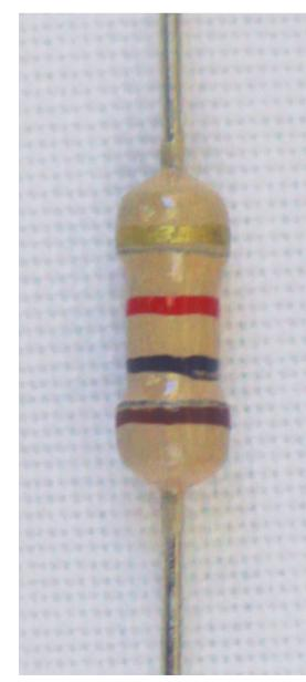
Figure 3: A typical resistor
