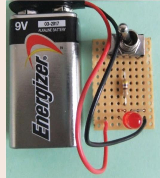
Figure 9: A simple LED circuit built on a strip board
