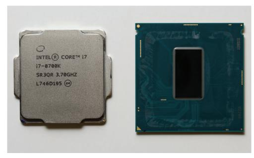
Figure 3.2: Intel Core i7 CPU
