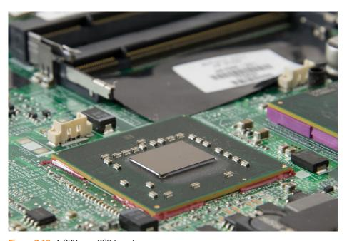
Figure 2.13: A GPU on a PCB board
