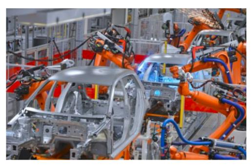
Figure 1.3: Robots welding in an automotive factory
