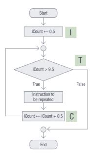
Figure 7.6: Coding and flowchart for a WHILE loop
