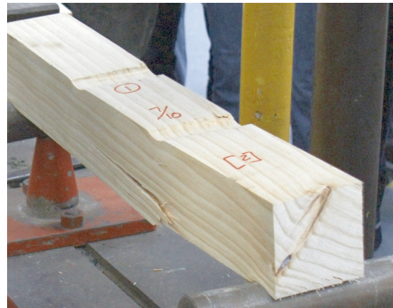
Figure 5.31b The square-section wood beam shows failure in tension at the bottom, splitting due to compression at the top and shear planes in the middle.
