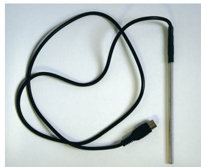
Figure 16.11e A temperature sensor containing a thermistor
